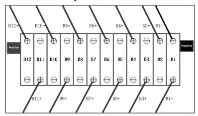
According to the wire label on the equalization subharness, B1 - is connected to the negative electrode of No. 1 cell (B1), B1 + is connected to the positive electrode of No. 1 cell (B1), B2 + is connected to the positive electrode of No. 2 cell (B2), and connected in sequence.
