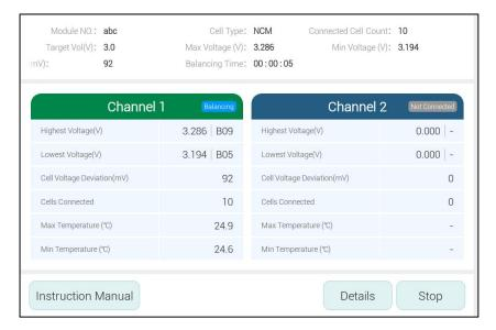
3) During the balancing process, you can check the test progress and wait for the test results. Click **Stop** to end the current balancing process.
