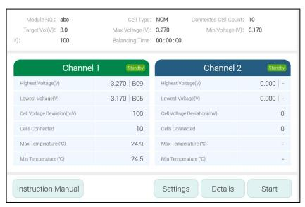
4) Click **Details** to view the specific data of the tested battery, including balancing time, cell voltage, cell balancing current, charge and discharge capacity, and temperature of each temperature monitoring point.
