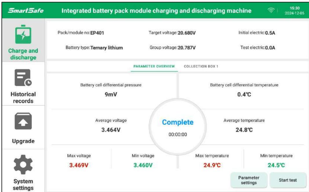
(4) If multiple 24CH sampling boxes are connected, you can click the corresponding sampling box to view the charging and discharging results of the battery module connected to it.
