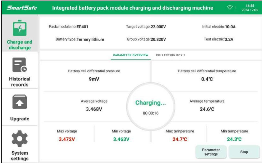
(3) During the charging and discharging process, you can check the test progress and wait for the test results. Click **Stop** to end the current charging and discharging process.
