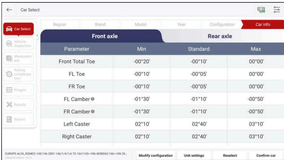
The screenshot shows the 'Car Select' screen with a table of standard vehicle parameters. The table is divided into 'Front axle' and 'Rear axle' sections. The parameters listed are Front Total Toe, FL Toe, FR Toe, FL Camber, FR Camber, Left Caster, and Right Caster. The values are given in degrees and minutes.
