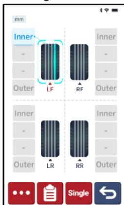
When conducting detection in single groove mode, the magnetic head of the detection equipment must be attached to the center of the groove, and then press the function button on the detection equipment to take measurements.
