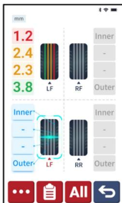
6. After completing the detection of all tires in sequence, the tire icon will be marked in different colors to indicate the detection results of the tire grooves.
