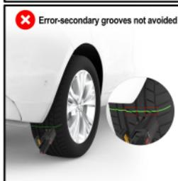
2. When conducting detection in all tread mode, the screen of the detection equipment must be facing the outside of the vehicle, as shown in the figure below.
