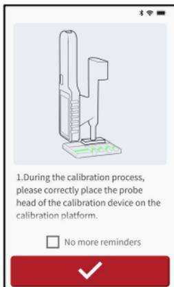
2. Press the function button on the detection equipment to start the calibration.
