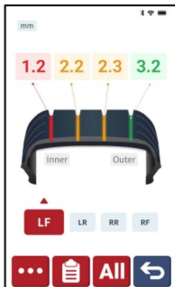
If a detection failure occurs, a pop-up will appear on the screen indicating measurement failed. Please confirm that the magnetic head of the detection equipment is in contact with the tire tread, and then press the function button again to re-measure.
