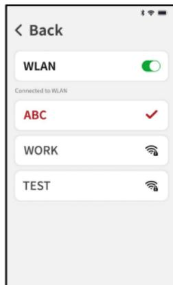
In the settings interface, click "**Network Connection**", then click the **WLAN** button, and the user can select the network they want to connect to. If the network name is displayed in red and is followed by "✓", it indicates that the connection has been successfully established.
