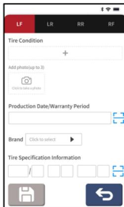
4. Click the tire name under the tire icon to select any tire for detection. After selecting the tire, attach the magnetic head of the detection equipment to the center of the tire tread, and then press the function button on the detection equipment to start the detection. At this time, the tire icon shows a scanning animation, while the laser window of the detection equipment emits a green laser.
