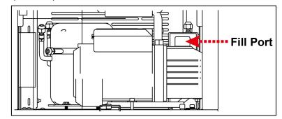
Note: the new vacuum pump oil cannot be filled too much into the vacuum pump otherwise it will spray out when working.
