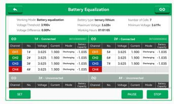
WEB1224 supports battery health status assessment, featuring a unique software algorithm to calculate SOC/SOH values. It automatically saves historical balancing records and supports two display modes: curve chart and bar chart.
