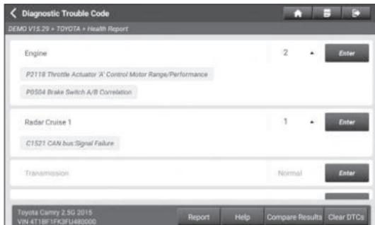
Systems with fault codes are displayed in red. Systems functioning normally are displayed in black.
