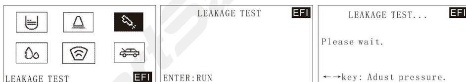
Leakage test is to inspect the sealing conditions of the injector needle valve under system pressure and to find out if the injector is dribbling.
