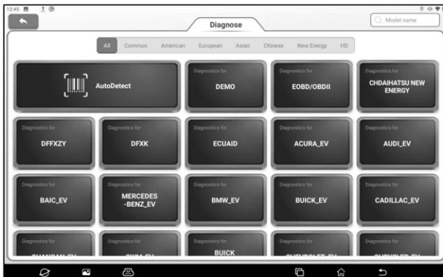
2. Click the vehicle brand to be tested to enter the model version information interface. Here we take Demo (Version 15.43) as an example to demonstrate how to diagnose a vehicle.
