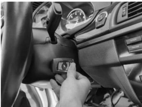
11. After the dealer key is successfully generated, please try to start the vehicle. Now the key matching is finished and the new key is ready for use.
