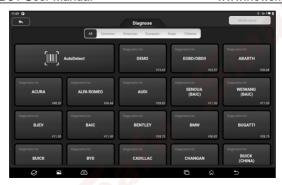
2. Click the vehicle brand to be tested to enter the model version information interface. Here we take Demo (Version 15.42) as an example to demonstrate how to diagnose a vehicle.
