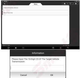
Note: If there is no anti-theft data of the target vehicle, select **Original Vehicle Key Obtained**, put the original vehicle key in the iSmartIMMO G3, and just follow the prompts to obtain it, no need to enter any data to complete the replacement.
