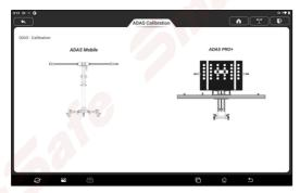
Tap the desired ADAS calibration tool (Take **ADAS Mobile** for example) to go to the next step.
