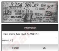
6. Tap **OK** to confirm the engine type and enter the function selection screen.
