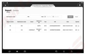
Note: To generate the test reports of different devices into a comprehensive inspection report, please enter the same maintenance number when saving the test reports of different devices.
