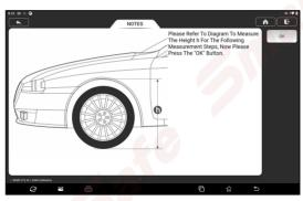
Follow the on-screen instructions to measure the height H (from the tire contact surface to the wheel housing edge) of each wheel respectively, and input the actual measured values.
