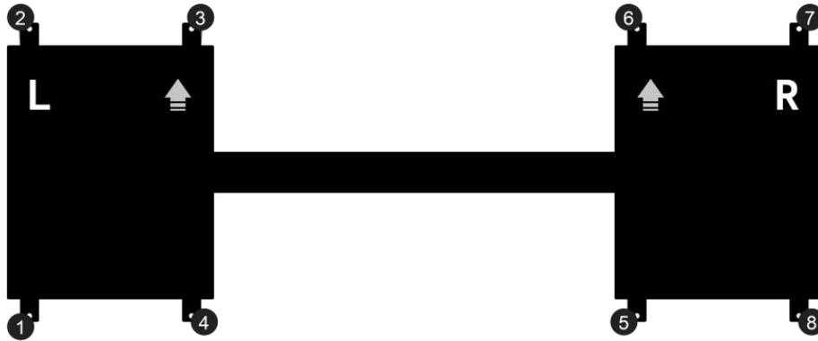
4. Place the left (L) and right (R) measuring units with reference to the installation positioning stickers, align the hole of the concrete anchor on the measuring unit with the ground, and then insert the bolt of the concrete anchor into the hole (as shown in the following figure at positions ① ~ ⑧).
