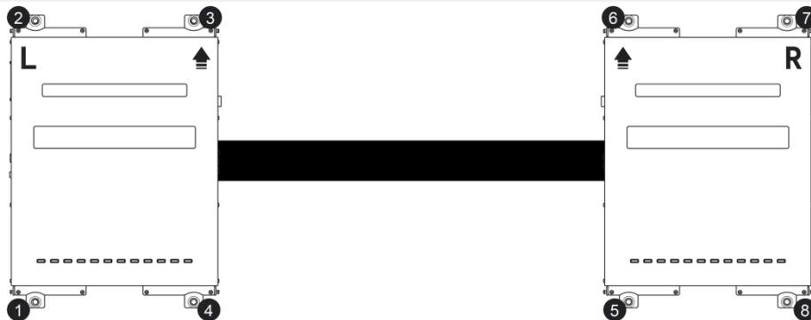
5. Take out the connecting bridge, unscrew the screws on the side (as shown in the figure below, there are 4pcs on each side), and remove the cover plate.
